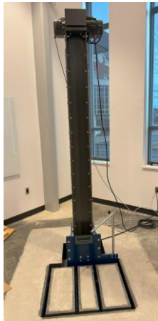
Lansmont PDT 300 Precision Drop Tester (661 lb maximum package weight, 41.5-in maximum dimension of package front-to-back, 1" to 72" drop height range)
