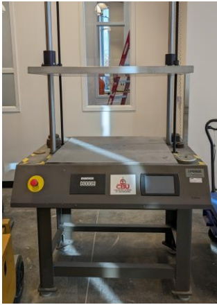
Lansmont Squeezer Compression Table (5000-lb capacity)
