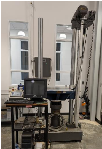
Lansmont Shock Tester Model 65/81 (500-lb capacity)
