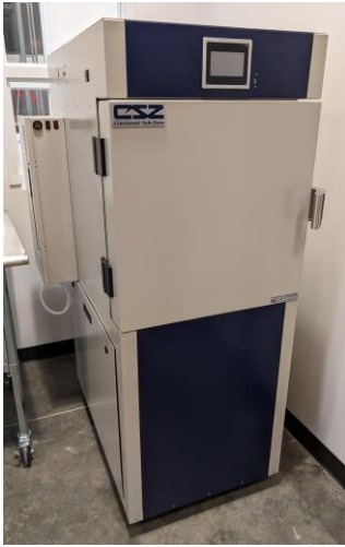
CSZ MCH-3-.33-H/AC MicroClimate with Humidity (3 CF test space volume, -85F to +375F temperature range, 10% to 95% RH range)
