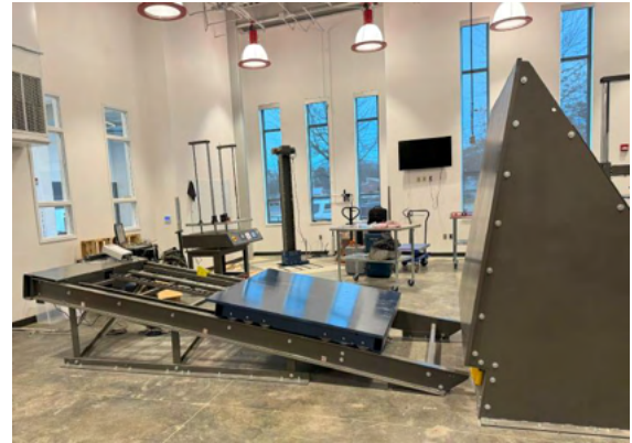
Lansmont 152-4K Inclined Impact Tester (60"x60" carriage size, 4,000 lb payload capacity, 7.3 ft/sec velocity)
