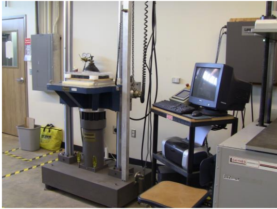
Lansmont Shock Tester Model 65/81 (500-lb capacity)
