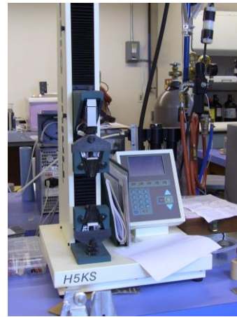
Hounsfield Materials Tester Model H5KS (Load capacity is 5kN with a speed range from 0.01 to 1000 mm/min)
