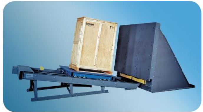
Lansmont 152-4K Inclined Impact Tester (60"x60" carriage size, 4,000 lb payload capacity, 7.3 ft/sec velocity)
