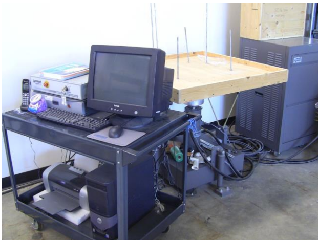
Lansmont Model 1000 Vibration Test System (75-lb capacity)
