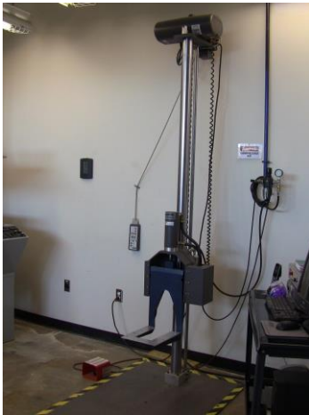
Lansmont PDT-56ED Drop Tester (175-lb capacity)
