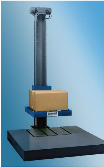
Lansmont PDT 300 Precision Drop Tester (661 lb maximum package weight, 41.5-in maximum dimension of package front-to-back, 1" to 72" drop height range)
