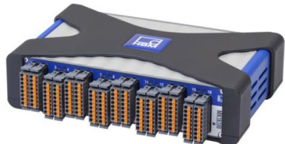
HBM QuantumX MX 1615B Strain Gauge Bridge Amplifier (16 channels with data rate up to 600 20kS/s per channel, full-, half-, or quarter-bridge 120 or 350 Ohm)
