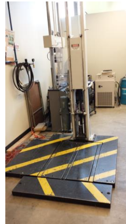
L.A.B. AD-500 Drop Tester (500-lb capacity)
