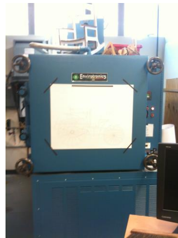
Envirotronics Altitude Chamber Model EA8-2-3-AC (-90F to +350F, Up to 100000 ft altitude, 24"x24"x24" chamber size)
