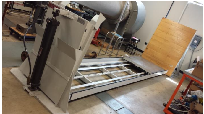
L.A.B. Incline Impact Tester (500-lb capacity)
